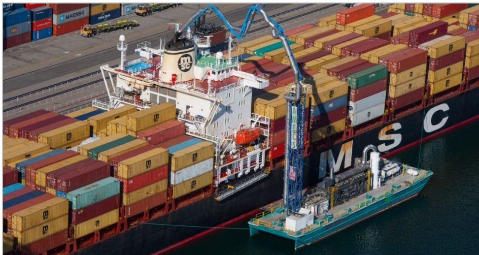
Figure IV.6-2. Barge-Based Emissions Control System 12
