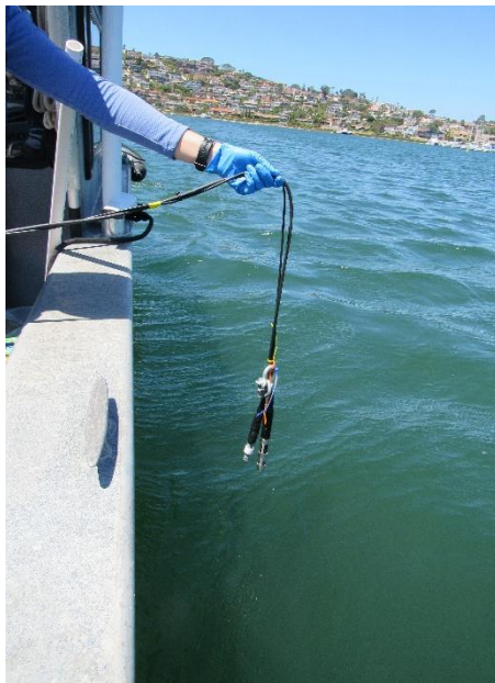
Photo A. Water quality readings of temperature, conductivity, salinity, pH, and dissolved oxygen are taken before, during, and after sampling using a YSI Pro Plus data sonde.
