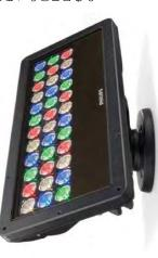
(36no) with a delivered light output of 2161 lumens when all Die cast aluminium housing with olear tempered glass lens, 6ft unified power/data cable and standard black power coated finish and supplied with integral DMX LED driver. distribution. Utilizing 120V 50W RGBW (4000K) LED array Exterior quality, UL Wet Location, IP66 and IK10 rated 10° collimated optical lenses for narrow beam optical bracket mounted colour change LED projector, with
