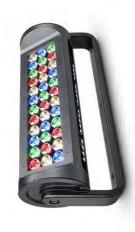
distribution. Utilizing 120V 100W RGBW (4000K) LED array (36no) with a delivered light output of 3251 lumens when all Die cast aluminium housing with clear tempered glass lens, integral male/femail waterproof connector and Standard black power coated finish and supplied with integral DMX LED driver. Exterior quality, UL Wet Location, IP66 and IK09 rated 5° collimated optical lenses for narrow beam optical stirrup mounted colour change LED projector, with LEDs are operational. Description:
