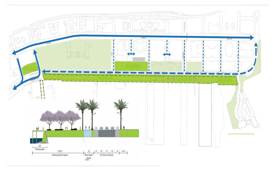
Potential Alternative No. 1 – Narrowed Harbor Drive (53') provides dedicated through traffic lane in North and South direction, a center turn lane, and provides parallel parking and loading zone on both sides of the street between G Street and Ash Street, and parallel parking and loading zones on the west side of Harbor Dr. and Diagonal parking on the east side of Harbor Drive between Ash and Grape Street.
