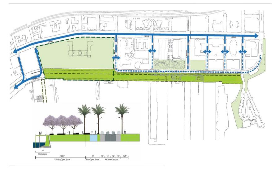
Potential Alternative No. 2 – Narrowed Harbor Drive (44') provides single lane of traffic in the north and south direction with parallel parking and loading zone on each side of the street. Proposed closure of Harbor Drive from Ash Street to Grape Street with a single lane adjacent to County Waterfront Park dedicated solely for emergency and service vehicles.
