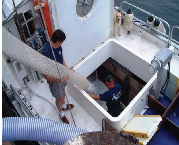
Fig 3.23 - Blowing ice into a vessel's hold – photo from <https://www.northstarice.com/catalog/product-applications/seafood>
