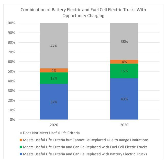
Although 4% of fuel cell truck trips may not meet the daily mileage requirement of trucks, with appropriate hydrogen refueling stations in place, these vehicles should be able to accomplish the operating demands of the trucks.
