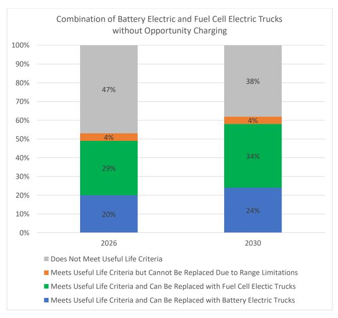
Although 4% of fuel cell truck trips may not meet the daily mileage requirement of trucks, with appropriate hydrogen refueling stations in place, these vehicles should be able to accomplish the operating demands of the trucks.
