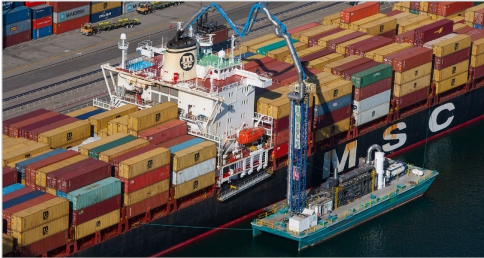
Figure IV.6-2. Barge-Based Emissions Control System 12
